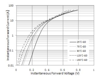
Figure 2. Typical Instantaneous Forward Characteristics
