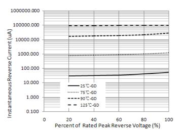
Figure 4. Typical Reverse Characteristics
