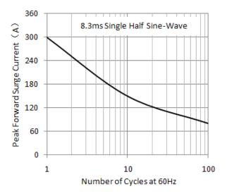
Figure 3.Maximum Non-Repetitive Peak Forward Surge Current
