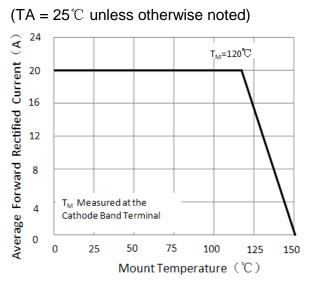
Figure 1.Forward Current Derating Curve
